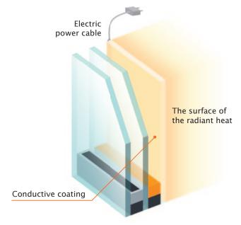
Heating glazing can not only compensate the heat losses in buildings, but also can become an alternative to traditional heating system.
